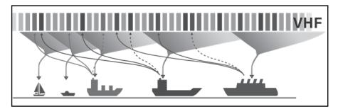
Figure 15. Frequency sharing in the AIS network uses self-organized time division multiple access. Source: AIS Reporter/used with permission
