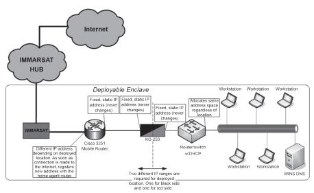
Figure G-5. Deployable Enclave with INMARSAT Connection
