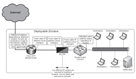
Figure G-4. Deployable Enclave with Direct Internet Connection
