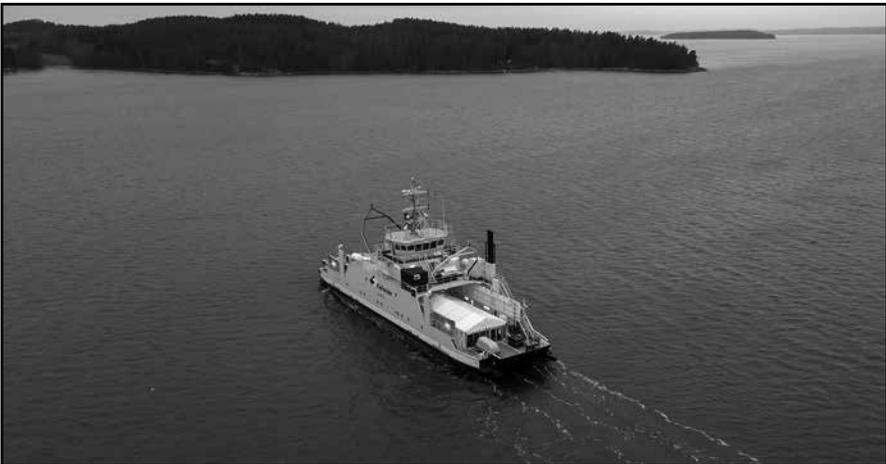
Figure 22. Demonstration of the first fully autonomous transit and docking of a vessel, using the car ferry *Falco*. Source: Finferries/used with permission
